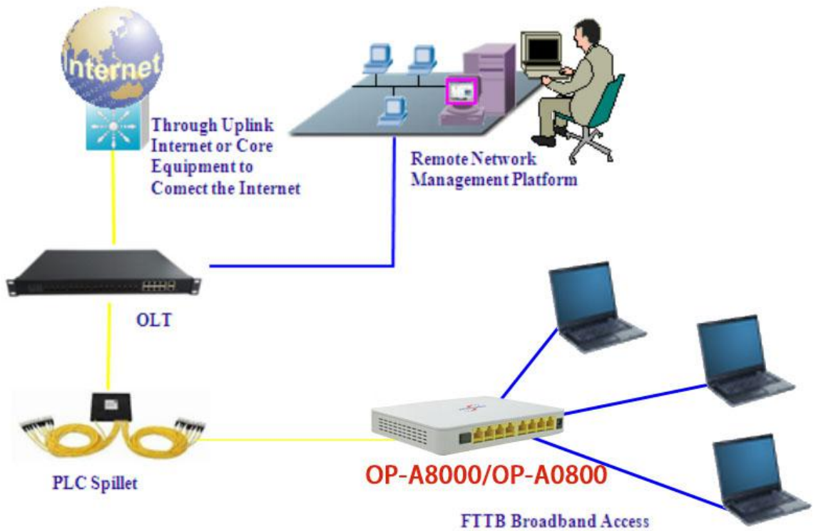
Figure: OP-A8000/OP-A0800/OP-A8000D/OP-A0800D Application Diagram
