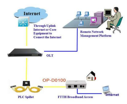
Figure: OP-D0100 Application Diagram
