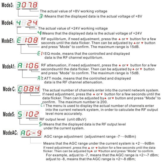
Note: AGC range per reduce 1 dBm, the output level is raised by 2 dBuV.
