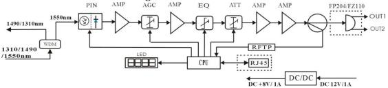
Note: The circuit in the dashed box is optional configuration circuit.
