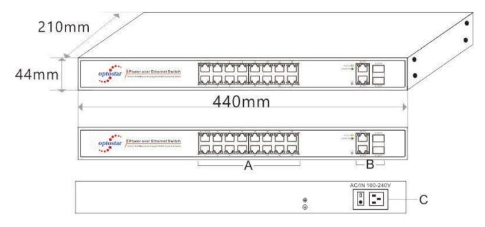
A.16 \* PoE Ports B. 2 Sets of Combo Port C.100-240VAC,50/60Hz
